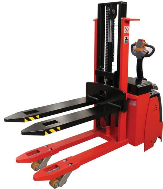
One SMART POWER UNIT is able to fully manage one lift from both hydraulic and electric point of view. It allows a consistent reduction of the TCO of the machine reducing assembly time since several sensors are embedded. It Integrates a wide number of I/O which can direct-drive valves both on-off or proportional.
