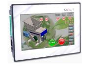
A Smart Power Unit is equipped with all the hydraulic, electric and electronic features required to fully manage a complete complex machine (see full data sheet). The electronic and mechanic architecture is developed in order to meet SIL 2 (safety integrity level) as per EN61508 for or PI c as per EN13849
